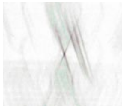
Figure 4 : General Hough Space. Indicates the likely presence of a shape at the center of the image
